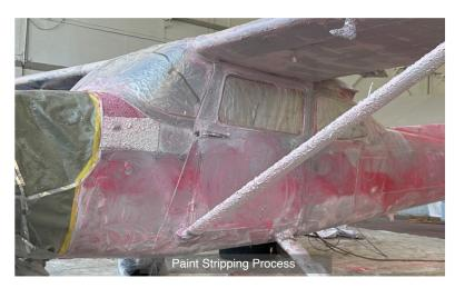
And with that done, the work begins. I won't bore you with every detail but it needs to be mentioned they go to great lengths protecting the windows, tape all the aircraft seams and protecting the engine during the paint stripping process. After that stage they strip remaining paint by hand around the windows and seams.
